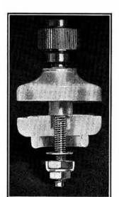
Twenty million of anything is a lot, 20 million megohms is the resistance of the new "Belling-Lee" high leakage resistance terminal specially designed for instrumentation in nuclear physics, triode electrometers, high resistance bridges, etc. A smaller type is available with a resistance of 3 · 6 million megohms. Tests were taken at 850 volts D.C. 55° F and 70% relative humidity.
